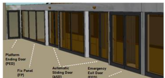
Fig. 2. Schematic drawing of PSD sliding door system
