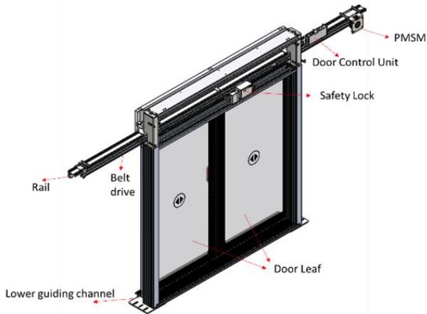
Fig. 3. Schematic drawing of PSD sliding door system
